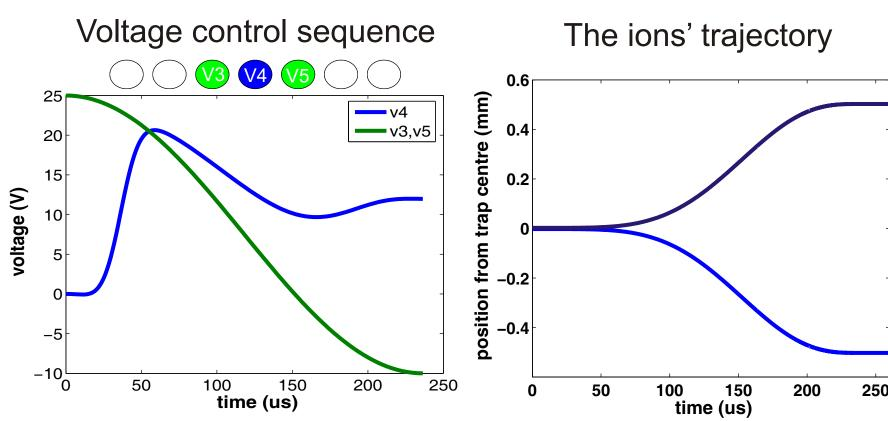
Separating ions at trap centre: Using symmetries the problem simplifies to a one ion movement process. This cannot be done when separating ions off-centre.
