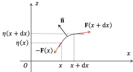
Tension forces give a resultant force  $d\mathbf{F} = \mathbf{F}(x + dx) - \mathbf{F}(x)$  which component normal to the surface element has to be balanced by pressure forces, as seen in section 2.3.3.
