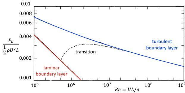
The figure shows the drag  $F_D$  normalized to  $\rho U^2 L/2$  as a function of the Reynolds number in a turbulent boundary layer.
