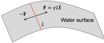
We consider a line of length  $L$  at the surface of the water. The molecules on one side of this line exert a pulling force (tension) on the molecules on the other side.
