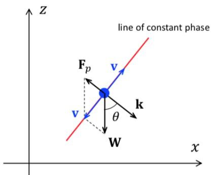
The figure illustrates the motion of a fluid element (represented by the blue dot). The pressure force  $\mathbf{F}_p = -\nabla p = -k p$  is perpendicular to the lines of constant phase and directed upwards (since pressure decreases upwards). The weight  $\mathbf{W}$  is downwards, and the resultant net force is along the line of constant phase, as this is the line along which the fluid element moves.
