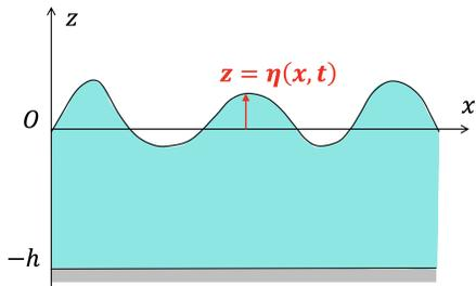
We consider two dimensional waves. The axis  $z = 0$  corresponds to the flat surface at equilibrium and the equation of the perturbed free surface is  $z = \eta(x, t)$ . The depth of water is  $h$ .
