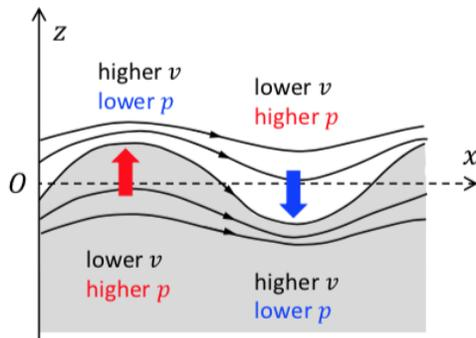
When the interface is perturbed, the streamlines are brought closer to each other above the crests and below the troughs, so that the flow velocity increases there (due to mass conservation), which implies that the pressure decreases (due to Bernoulli's theorem).
