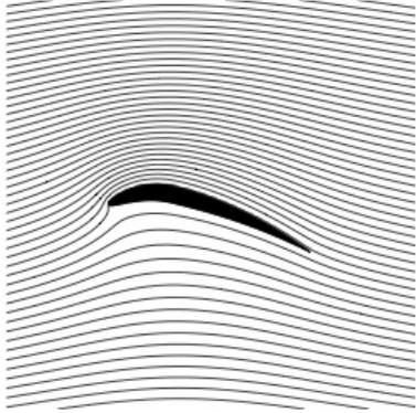
As illustrated on the figure, this aerofoil gives a much larger lift than a symmetrical aerofoil. The lift is also larger if the aerofoil is thinner, which is why birds have thin wings. Airplanes however tend to have thicker wings because there are other considerations coming into play, such as design and fuel storage.
