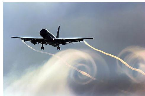
It is the bound vortex that creates the circulation around the wing required to produce a finite velocity at the trailing edge and which results in a lift. Note that although a vortex
