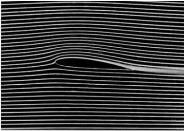
Therefore, the flow *behind* the plate also has vorticity. It is called the *wake*. It can be seen together with the boundary layer on the figure which shows streamlines around an aerofoil immersed in a fluid.
