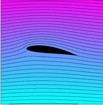
The figure shows the streamlines relative to a Joukowski aerofoil which is inclined with respect to the oncoming flow. (Credit: Wikimedia)
