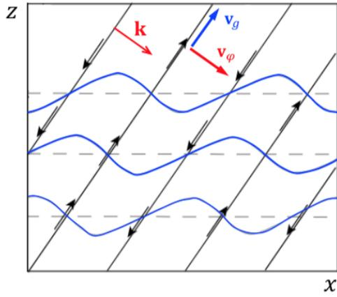
The figure illustrates the motion of fluid elements and propagating internal gravity waves.
