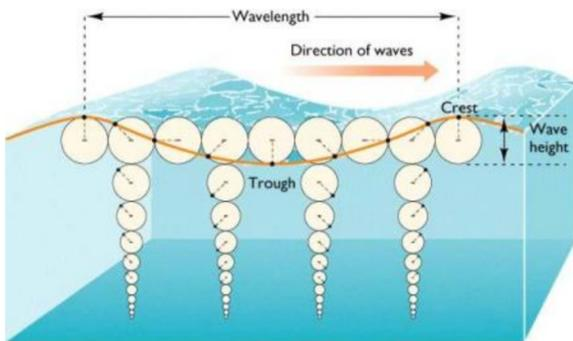
The figure illustrates the path of fluid elements displaced from their equilibrium position. The radius of the circles decreases exponentially with depth.
