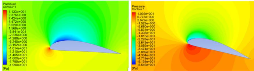
The pressure is maximum at the edges, where there are stagnation points, and has a minimum on the upper side. Therefore, *we expect the boundary layer to separate at some point along the upper surface of the aerofoil*, and separation occurs closer to the leading edge for higher angles of attack.
