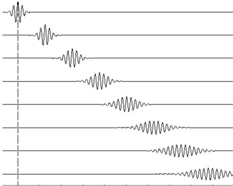
The figure below shows a wave packet traveling in the  $x$ -direction. Dispersion results in a flattening and broadening of the envelope.
