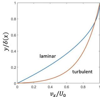
Therefore, vertical mixing is much more efficient in the turbulent case, and the flow is accelerated much more efficiently through the boundary layer, as shown by the velocity profile on the figure. (Credit: <https://aerospaceengineeringblog.com/boundary-layers/>)
