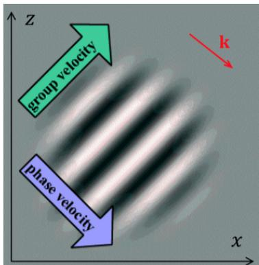
In other words, the envelope of wave packets and the energy propagate in a direction which is perpendicular to the direction of propagation of the crests and troughs, as illustrated on the figure.
