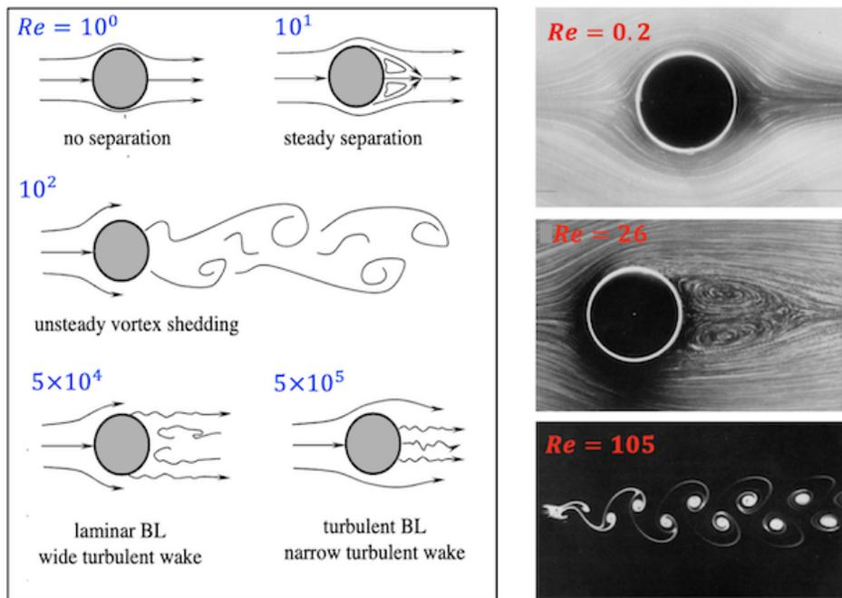
What is seen at  $Re = 105$  is called a *von Kármán vortex street*. It appears when vortices are emitted alternatively by the flow on top and on the bottom of the object. The emission is periodic. This leads to a lift on the cylinder which oscillates with time. In a realistic set up, when the frequency of the oscillation matches some natural frequency of the object, structural damage to the object may occur<sup>2</sup>.
