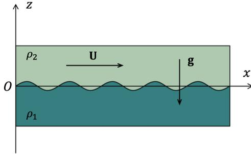
The interface between the two fluids is perturbed such that its equation becomes  $z = \eta(x, t)$ , with  $\eta$  being the real part of:
