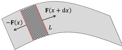
We now consider the forces exerted on the dashed surface element which is between  $x$  and  $x + dx$  and for which the length  $L$  is along the  $y$ -axis.
