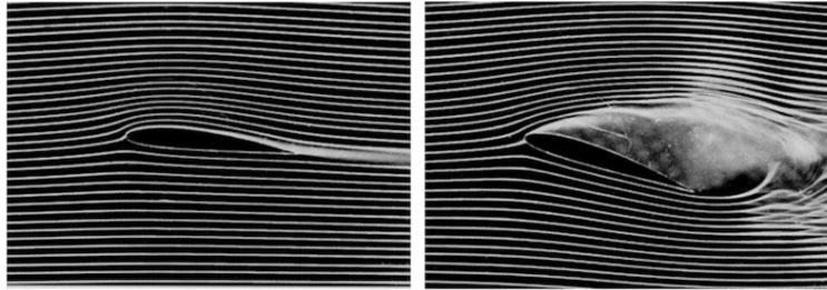
Delaying boundary layer separation is therefore a major goal in the design of airplanes or fast vehicles. This can be done by streamlining the aerofoil (or any fast vehicles), that is to say by aligning its back surface with the unperturbed streamlines of the outer flow. That is why many sea mammals or fishes have tapered caudal fin shaped like a crescent moon.
