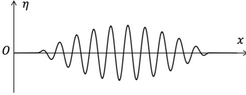
We assume that the coefficients  $a(k)$  are non zero only in a narrow interval of wavenumbers centered on  $k_0$ . Such a disturbance is called a *wave packet* and is represented on the figure.
