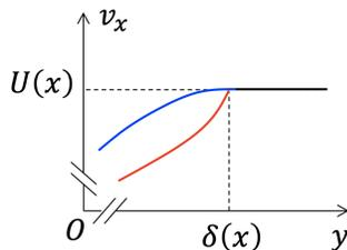
At the surface  $y = \delta$  of the boundary layer,  $v_x$  matches the velocity  $U(x)$  of the outer flow. For the stress to be continuous at  $y = \delta$  (and therefore volume forces to stay finite),  $v_x$  has to approach  $U(x)$  following the blue curve and not the red curve.
