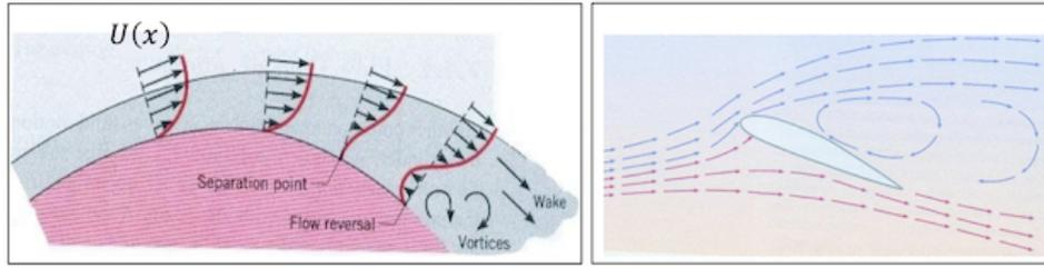
When separation occurs, Prandtl's equation (4.9) does not apply anymore, as  $v_x$  is no longer very large compared to  $v_y$ . In fact, separation occurs at the point where this equation becomes singular (see Landau & Lifshitz, Chapter IV, §40, for more details).
