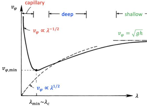
This figure shows the phase velocity  $v_\phi$  as a function of wavelength  $\lambda$  for the different type of surface waves mentioned above. The phase velocity has a minimum for  $\lambda \sim \lambda_c$ .
