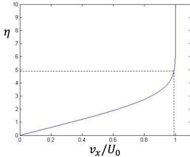
This boundary value problem has to be solved numerically. The figure shows the solution obtained for  $v_x/U_0$  as a function of  $\eta = y/\delta(x)$ . The fact that  $v_x/U_0 = 0.99$  at  $\eta = 4.9$  confirms quantitatively that  $\delta(x)$  gives a measure of the thickness of the boundary layer (this had been obtained by a qualitative argument only in section 4.1.1).
