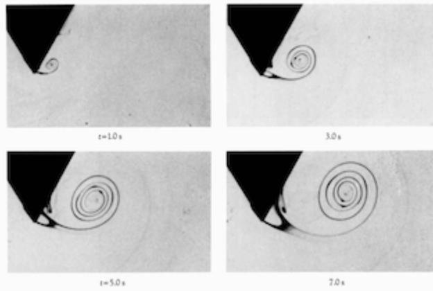
From Van Dyke, *Album of Fluid Motion*. The figure shows a starting vortex produced when a viscous fluid is moved impulsively past a wedge.
