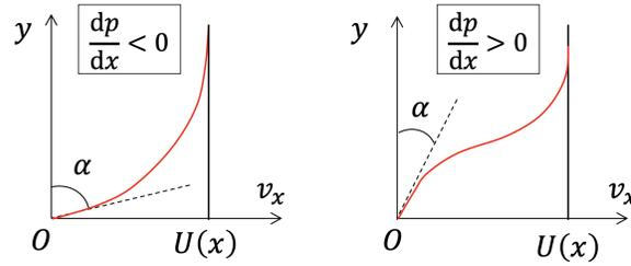
The fluid near the rigid boundary is subject to the following forces: (i) it is decelerated by the frictional force from the boundary, (ii) it is accelerated by the viscous stress from the upper layers, that is to say by the transfer of momentum from the outer flow which moves at velocity  $U(x)$ , (iii) it is accelerated or decelerated by the pressure gradient, depending on whether it is negative or positive.
