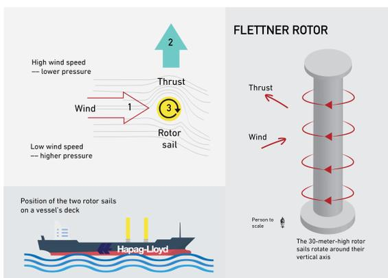
This figure illustrates how the Magnus effect can be used on a ship to reduce fuel consumption.
