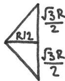
$$\begin{aligned} A_2 &= \frac{1}{2} \times \sqrt{3}R \times \frac{R}{2} \\ &= \frac{\sqrt{3}R^2}{4} \end{aligned}$$
