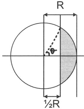
$$\begin{aligned} \text{Shaded area} &= \text{Sector} - \text{Triangle} \\ A &= A_1 - A_2 \end{aligned}$$
